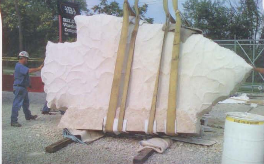
The 15' X 9' X 2' arrowhead crafted for the entrance to the practice facility of the Kansas City Chiefs football team is ready to be moved by crane. To fabricate the piece, Middlemas and apprentice Gregg Mohr worked on one side, then had the stone flipped.
